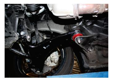
Install the vertical bushing with P/N 03P03638 up. Only grease the leading edge to help get the bushing started. DO NOT grease the I.D. of the bushing when installing the inner sleeve.
